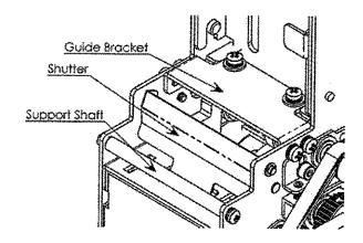
The card should be able to slide freely under the Shutter. For optimum operation, the bottom of the Shutter should be positioned no more than card thickness +0.2mm above the Base Plate.
